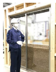
Shutter - lateral pressure verification using reproduced snowfall
