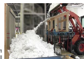
Shutter - lateral pressure verification using dummy materials simulating snow accumulation
