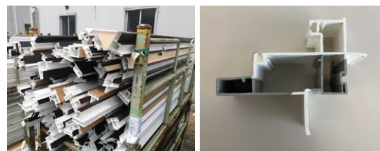
(Left) Vinyl scraps produced during vinyl window manufacturing. (Right) A vinyl profile made from reused vinyl scraps (gray parts are recycled materials)
