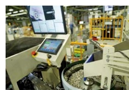
600 million screws manufactured annually, all inspected with our 100% inspection system
