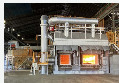
Recycling furnace at the Shikoku Plant. At the back left is an automatic material feeder
