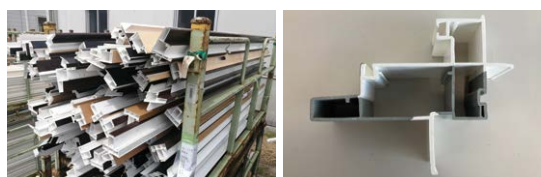
Left: Vinyl scraps generated during the vinyl window manufacturing process. Right: A vinyl profile made from reused vinyl scraps (gray parts are recycled materials)
