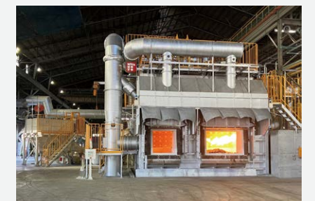
Recycling furnace at the Shikoku Plant. At the back left is an automatic material feeder
