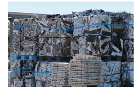
Aluminum, also known as "electricity in a can," requires a large amount of electricity for electrolysis to refine it from raw materials such as bauxite. However, because aluminum can be remelted using only a small amount of energy, aluminum recycling plays a very important role in reducing CO 2 emissions.
