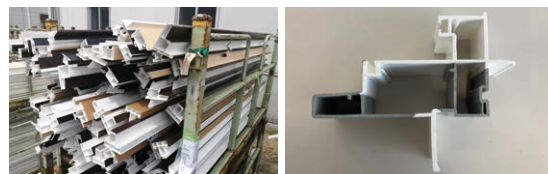
Left: Vinyl scraps generated during the vinyl window manufacturing process. Right: A vinyl profile made from reused vinyl scraps (gray parts are recycled materials)
