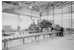
Aluminum extruder installed in 1959
