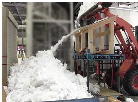
Shutter side pressure verification using reproduced snowfall
