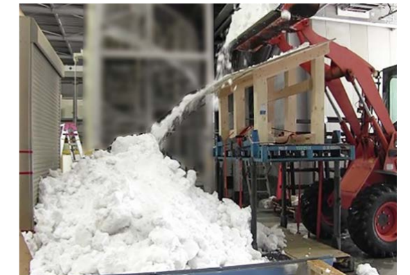
Shutter side pressure verification using reproduced snowfall
