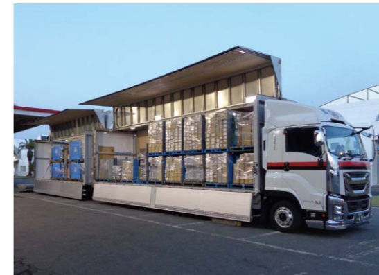
Unit loading facilitated by the introduction of the proprietary Y-Caps system
