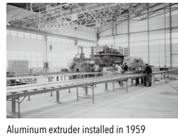
Aluminum extruder installed in 1959
