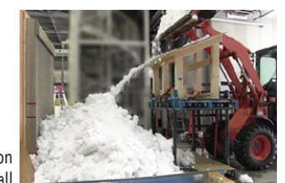
Shutter - lateral pressure verification using dummy materials simulating snow accumulation
