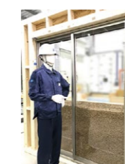
Shutter - lateral pressure verification using reproduced snowfall
